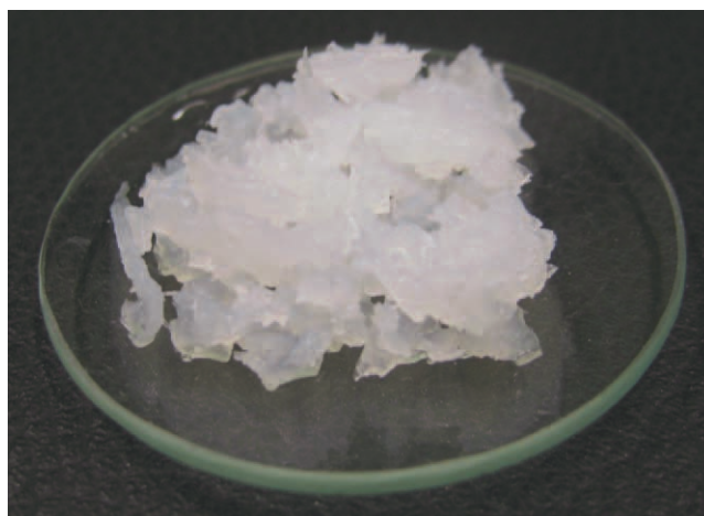
Figure 1 Picture of hydrated GELPEO lumps after dialysis. [Color figure can be viewed in the online issue, which is available at wileyonlinelibrary.com .]
